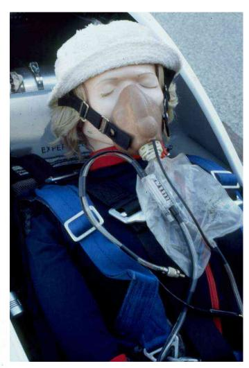
This picture shows the Nelson A4 flow regulator. Notice the two scales, the right is 0-25 or 25,000 feet (7,500m) and is calibrated for a flow of 1 l/min/10,000 feet (3,000m). The left scale is similar to that used with the conservation cannula. The sierra mask system is as efficient as the conservation cannula, probably even more so, but is designed to be used above 18,000 feet (5,500m).
