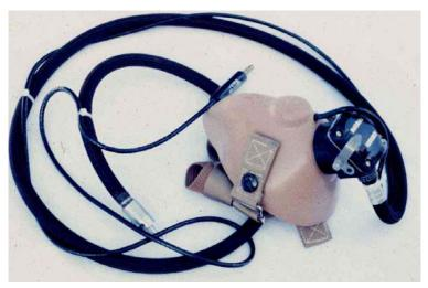
This interesting system is called the Altox system. It uses a pressurized supply between 20 and 60 pounds per square inch. The black body attached to the nose of the mask is a regulator which is sensitive to mask pressures produced by breathing. It is not very efficient in that it requires constant oxygen except for a small blend hole on the side by the silver lever. I am interested in paperwork and documentation on this unit. Unfortunately, to this date I have not
