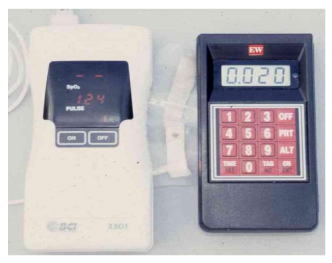
Today the measurement of oxygen saturation and altitude is much easier. This little oximeter on the left can be put in a pocket and the barograph on the right is of similar size. Each will record into memory the flight data. The data only needs to be down loaded and matched for time
