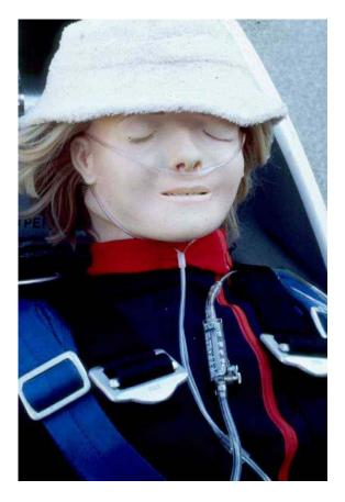
Mountain High of Salt Lake City to the rescue. Patrick McLaughlin has developed this handy dandy EDS (Electronic Delivery system) oxygen regulator for use with the standard cannula. Basically, it monitors your breathing by measuring pressure changes at your nostril and when it determines the beginning of inspiration, gives
