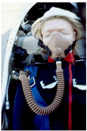
surplus. It is a system which will blend oxygen based upon altitude and then begin to increase pressure against exhalation (breathing out) in order to maintain sufficient oxygen pressure in the lungs. It is not automatic. Here the regulator is located
