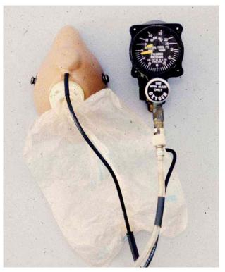
Another frequently used method of regulating the oxygen flow is the A8 regulator. Also an Air Force hand me down, these regulators are very susceptible to mal adjustment and flow errors. Frequently, these units are red tagged by a maintenance shops, thus becoming paper weights. Their advantage is that they are easily adjustable with a readout in thousands of feet.
