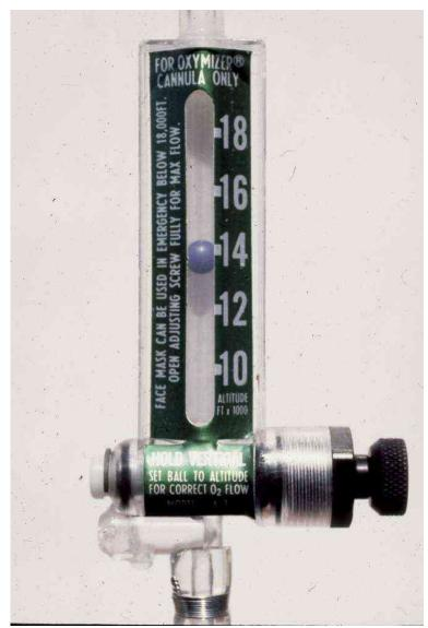
The flow meter on Annie's chest produces flows of about 500 ml/min/10,000 feet (3,000m), and is calibrated up to 18,000 feet (5,500m) as determined by the numbers on the right side.
