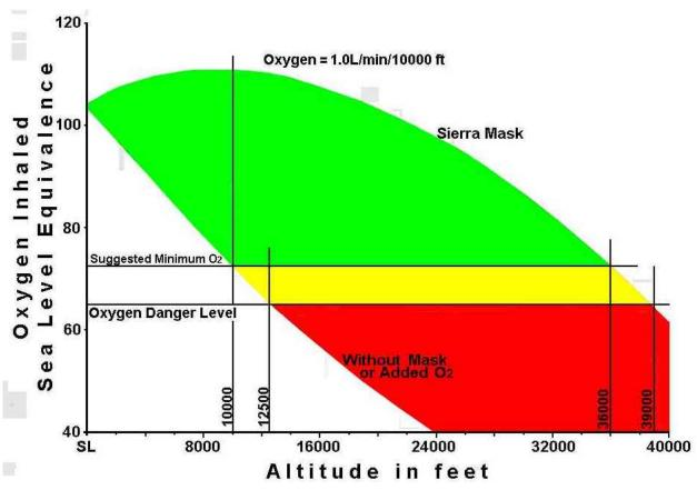
10,000 feet (2,700-3,000m) and the red range at 12,500 feet (3,750m). In contrast, the sierra mask when used correctly, enters the caution range about 36,000 feet (11,000m) and the danger area at about 39,000 feet (12,000m). I have personally used this system over 37,000 feet (11,500m).
