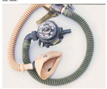
This is the venerable A14 system. As I mentioned before, surplus military units. On the face is a dial to change the oxygen concentration and back pressures so that it can be used to 44-45,000 feet (13,500m). Above 39,000 feet (12,000m) the unit produces resistance to exhalation so that in the low 40 thousands it is somewhat difficult to breath. It is like trying to breath with an air compressor in one's mouth.
